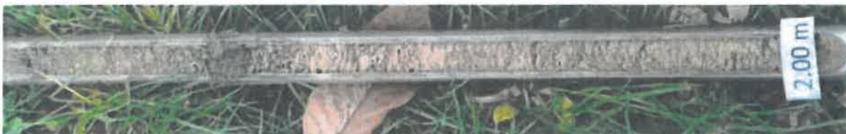
Figura 3.3. Prelevare probe cota -2.00m
